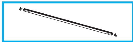
Slide four threaded sleeves into the cross bar's bottom channel and two into the top channel.
