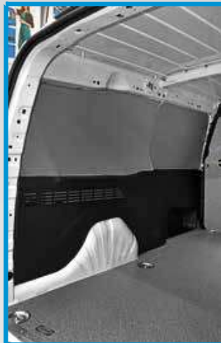
Berlino/Partner/Combo/Proace City 2018 L2: Floor and bulkhead liners in marble-look birch plywood, bodywork liners in grey prepainted steel sheet
