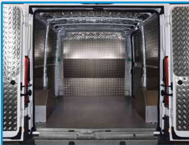
Ducato/Boxer/Jumper 2006/Movano 2022: Floor liner in marble-look beech plywood, bodywork and bulkhead liners in aluminium tread plate, wheel arch covers in aluminised steel sheet and aluminium tread plate
