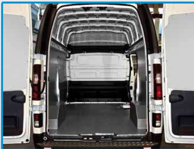
Vivaro/Trafic 2014/Talento 2016/NV300 H1: Floor liner in marble-look beech plywood, bodywork liners in grey prepainted steel sheet, wheel arch covers in aluminised steel sheet and aluminium tread plate
