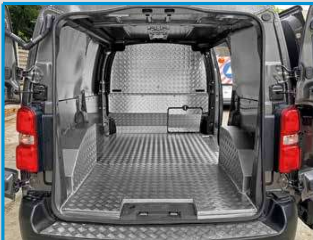
Expert/Jumpy/Proace 2016/Vivaro 2019/Scudo 2022 L2 H1: Double-layer floor liner in 9 mm birch plywood and aluminium tread plate, bodywork liners in aluminium, bulkhead liner in aluminium tread plate, wheel arch liners in aluminised steel and aluminium tread plate
