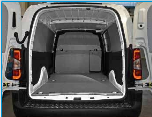
Berlino/Partner/Combo/Proace City 2018 L2: Floor and bulkhead liners in marble-look birch plywood, bodywork liners in grey prepainted steel sheet
