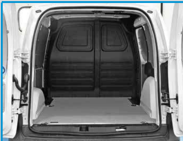
Kangoo/Citan 2021/Townstar 2022: Wooden flooring rubberized, side lining in painted metal sheet
