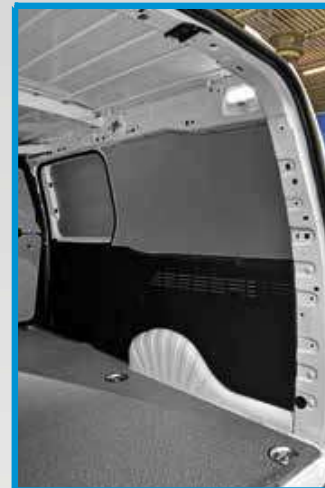
Berlino/Partner/Combo/Proace City 2018 L2: Floor and bulkhead liners in marble-look birch plywood, bodywork liners in grey prepainted steel sheet
