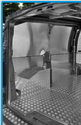
Expert/Jumpy/Proace 2016/Vivaro 2019/Scudo 2022 L2 H1: Double-layer floor liner in 9 mm birch plywood and aluminium tread plate, bodywork liners in aluminium, bulkhead liner in aluminium tread plate, wheel arch liners in aluminised steel and aluminium tread plate
