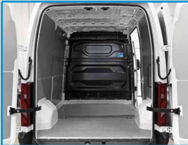
Master 2024: Floor liner in marble-look beech plywood, bodywork liners in grey prepainted steel sheet
